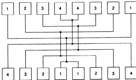
Fig. 5. Common-centroid layout of the storage capacitors.
